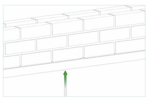
Use an HSS bit to drill and countersink an appropriate sized fixing hole through the frame. Insert sealant to fixing hole, then screw preferred fixing in place. Repeat process along the top track, ensuring fixings are within 900mm intervals.
