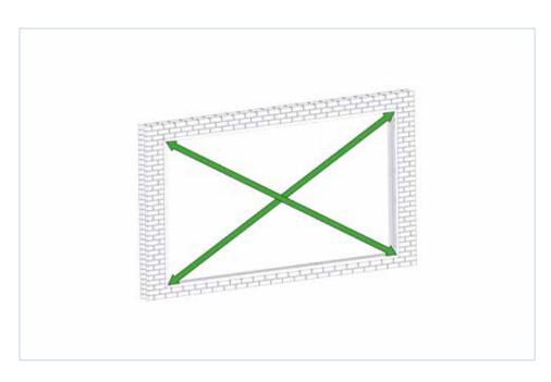
Measure diagonally from corner to corner to check the frame is square.
