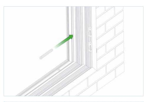
Screw preferred fixing in place. Repeat process along the jambs, ensuring fixings are within 600mm intervals.
