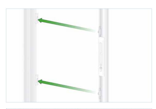
Align centre keeps with corresponding locking points (situated directly above and below handle).
