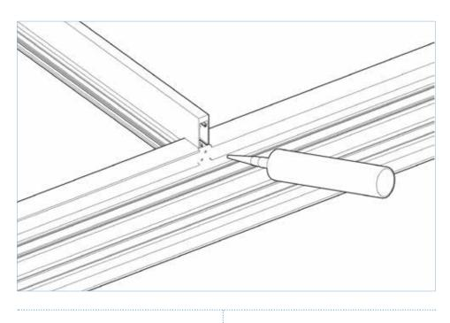
Seal holes with a suitable sealant.
