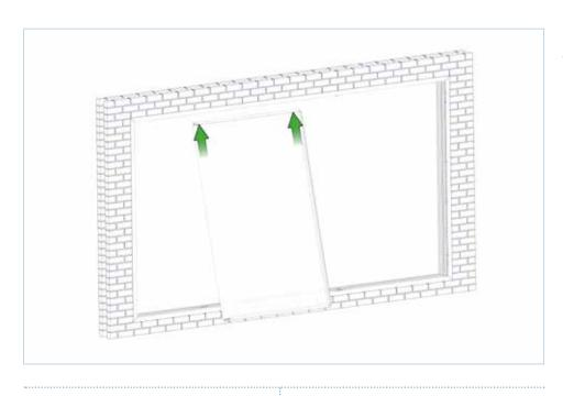
Insert top of sash into top track channel.
