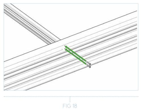
Fix interlocker in place with 3.9 x 16mm screws. Repeat process at both ends of profile.
