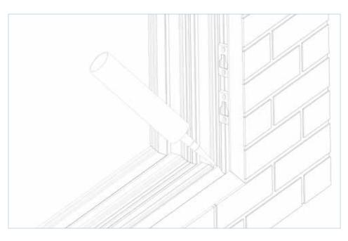
Seal the drainage isolator in place, ensuring ends of profile are sealed with edge of frame.
