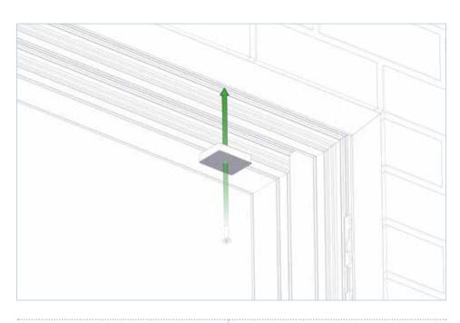
Fix anti-lift blocks above each sash corner when the sash is in the closed position. Fix using 3.9 x 25mm screws and position no more than 60mm from the external corner of the sash.
