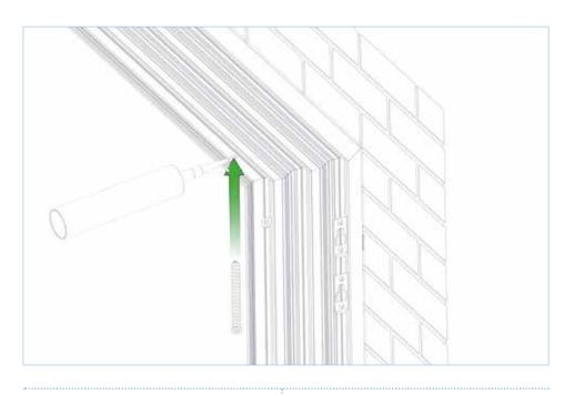
Insert suitable sealant to fixing hole, then screw preferred fixing in place. This must be done at both ends of the top track.
