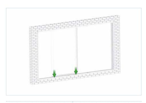
Drop sash on to running gear, ensuring the running gear sits within the bottom of the sash.
