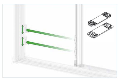
Working from bottom to top, adjust keep positions if necessary. Keeps can be packed out using the 0.5mm and 2mm packers supplied. Adjust keeps until the handle engages correctly, and the key in the lock cylinder turns smoothly.
