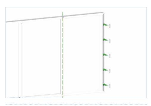
Use a straight edge or long level along the fixed interlocker to ensure straightness. Pack out accordingly between edge of glass and jamb.
