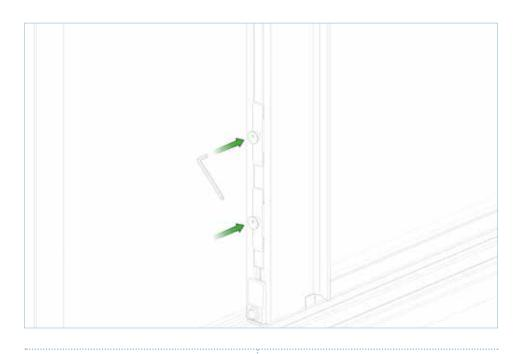
If more adjustment is required, use a 3mm Allen Key to adjust the locking point.
