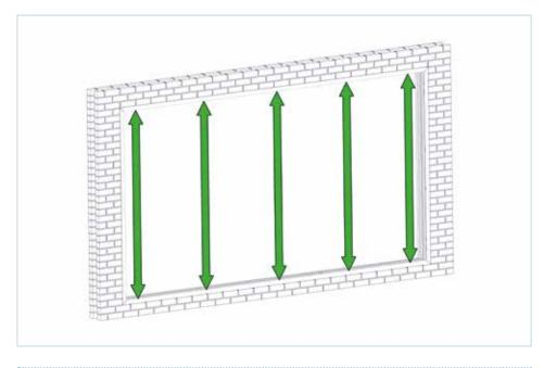
Accurately measure the internal frame dimensions.
