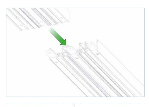
Connect the frame profiles together.
