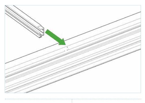
Align flush fixed interlocker to notch on bottom track. Ensure profile position is as per sections above.
