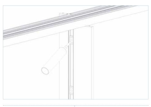
Apply supplied structural sealant around each packer.
