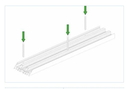
Where possible, fixing points should be on both sides of the frame, in a zig-zag pattern.
