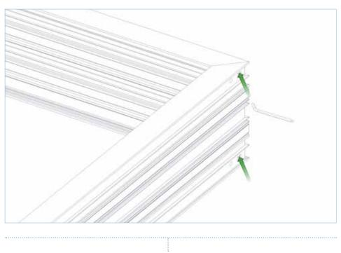
Tighten the cleat join with a 4mm Allen Key and screws provided.
