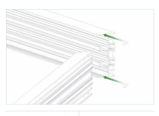
Insert alignment cleats to the frame. If set includes a fixed panel, one alignment cleat is required per corner and should be fitted in 25mm rebate.
