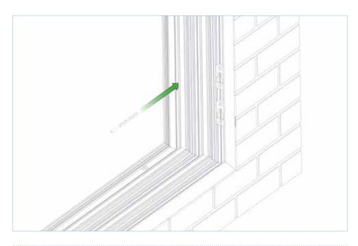
Use an HSS bit to drill and countersink an appropriate sized fixing hole through the frame. This should be no more than 150mm from the external corner of the frame.
