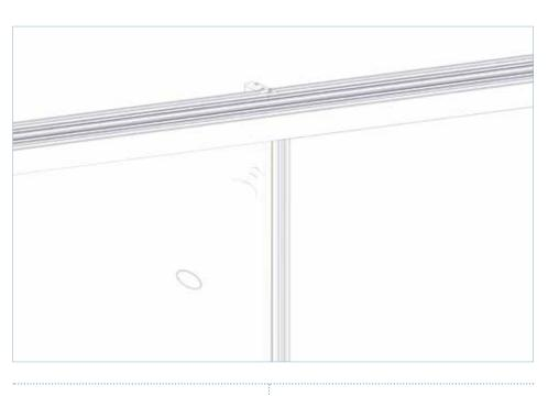
Apply bead of structural sealant along the length of interlocker (both inside and outside faces). Leave to fully cure before operating the set.
