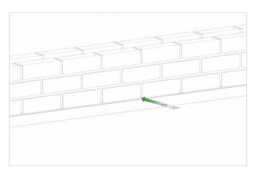
Pack out across the top track for consistent internal frame sizes. Ensure the track doesn't bow in any direction.
