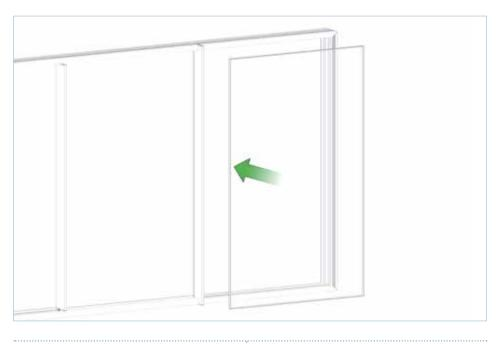
Insert glass into frame and slide over on to pre-applied structural sealant in interlocker. Pack out below glass, so it is central in the frame.
