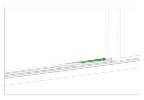
Fit wedge gasket between glass and outer frame, on both inside and outside glass faces.
