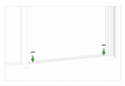
Place 10mm anti-lift packers into track channel.
