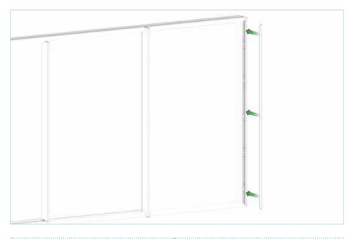
Secure frame bead in place. First clip top and bottom of bead, then proceed to clip in the centre.
