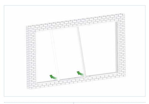
Swing bottom of sash above running gear.
