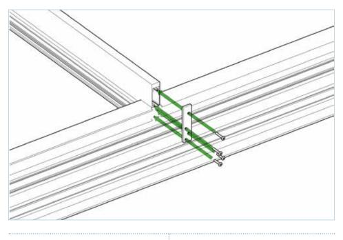
Fix interlocker end plate with 3.9 x 16mm screws. Repeat process at both ends of profile.
