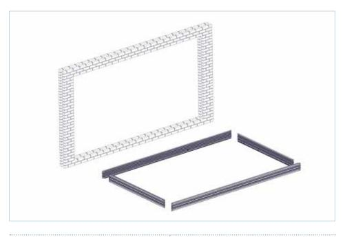
Lay frame profiles in front of aperture, being careful not to scratch the powder coat.
