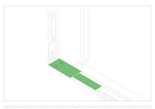
Check to ensure bottom of sash and running gear components are flush at both ends.
